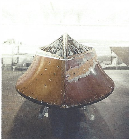
Riva boat stripped for restoration
